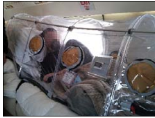
IsoArk N 36 series single person transport chamber
